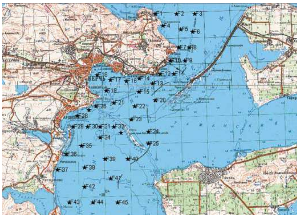
Fig. 8.4b. Scheme of the bottom sediments visual diving survey and sample collecting conducted in the Kerch Strait on 13–25 August 2008.
